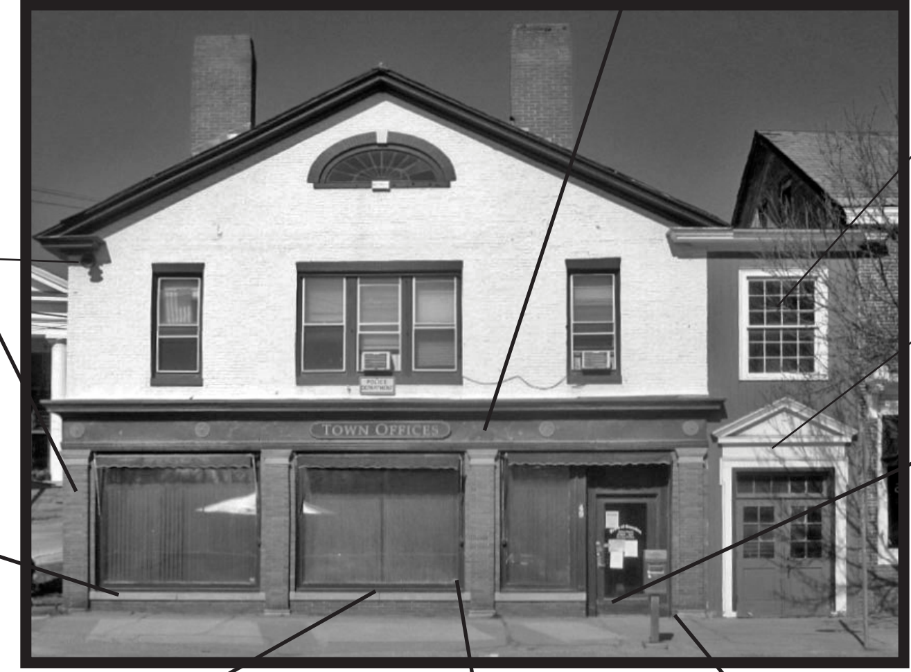
REPAIR EXISTING WINDOW AND REMOVE OLD WIRING - ADD NEW EXTERIOR ELECTRIC RECEPTACLES - SEE ELEVATION AND ELECTRICAL
