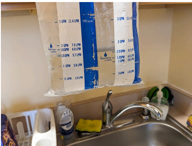
1.5 GPM Measured Flow at the First Story
