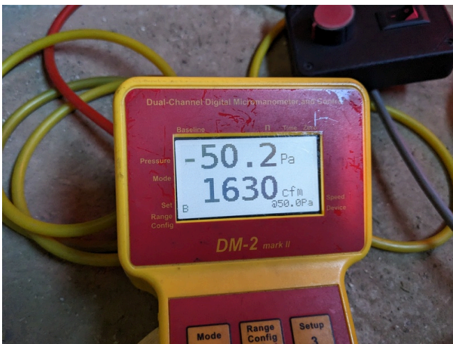
Building 5 - Blower Door Results
