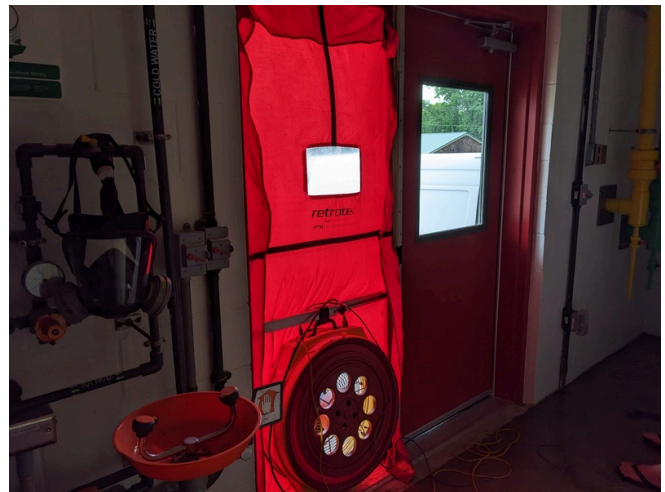
Building 3 - Blower Door Setup
