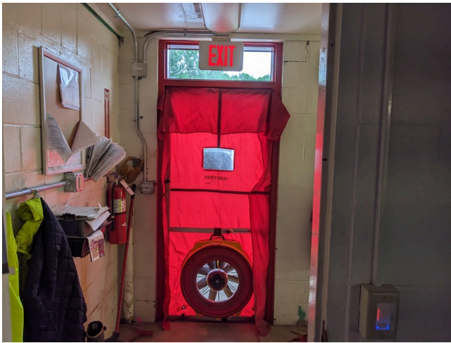
Building 2 - Blower Door Setup
