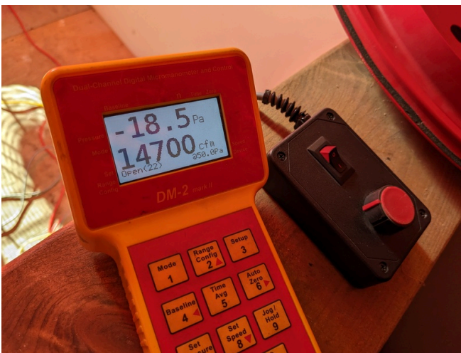
Blower Door at -18.5 PA
