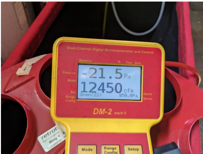
Old - Final Result; Old Building 2 Cannot Be Depressurized
